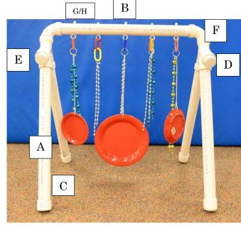
Purchase a 10 foot long piece of PVC pipe 1 ½ inch diameter and cut into five equal pieces each 24 inches in length. (This will make up the four legs and one center piece. (A & B) You can make the legs longer if you would like the mobile to be taller. Use sandpaper to smooth cut surfaces.
